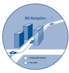
Adding an Inertial Navigation System allows us to determine orientation and navigate without access to satellite signals
